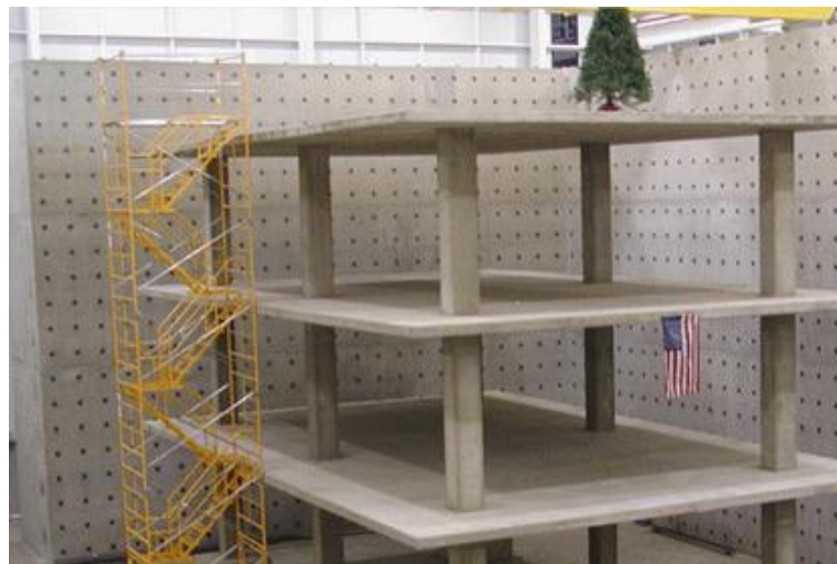
Fig. 1.13 Flat plate structure
