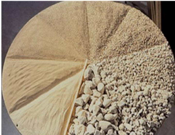
Fig. 9.1 Aggregates in Concrete
