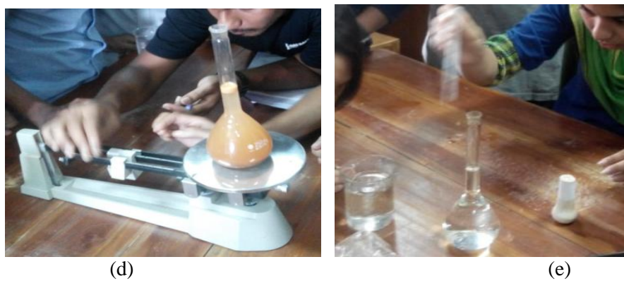
Figure 2.1: (a) Weight a blank pycnometer (b) Fill the pycnometer with 50gm soil and take weight (c) Fill the pycnometer with water up to mark along with soil and use vacuum pump to remove voids. (d) taking weight of soil and water with pycnometer (e) Fill the pycnometer with only water up to mark and take weight
