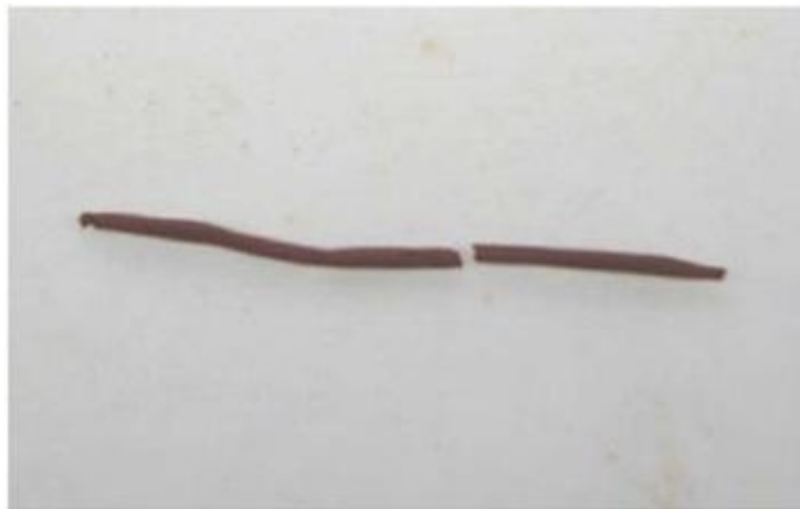
Figure 7.5: (a) Ellipsoidal Soil Mass (b) Soil Rolling (c) Soil Gets Crumbled at 1/8 inch (B.Sc. Eng. Thesis, Zakia Tasnim)
