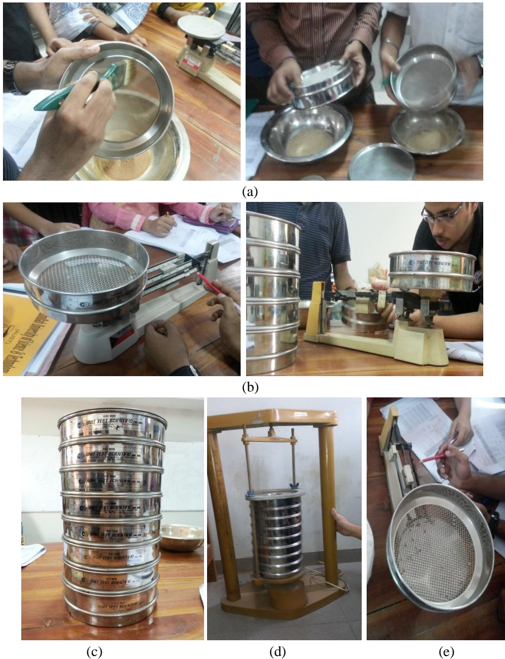
Figure 3.1: (a) Clean all sieves before test. (b) Weight all sieves (c) Serially set all sieves according to their opening size. (d) After pouring the soil place it to sieve shaker and shake 10 min. (e) Weight all sieve with contained soil
