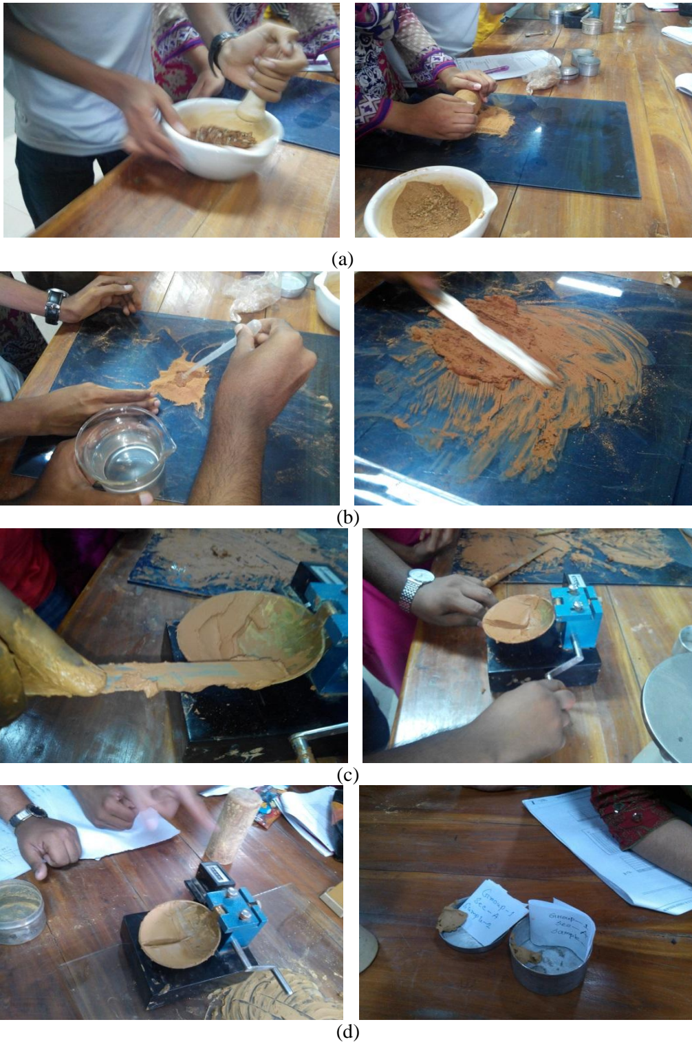
Figure 7.4: (a) Grind the soil sample into pieces (b) Mix considerable amount of water with the soil and make a paste (c) Using the spatula place soil sample to the liquid limit device, cut the soil sample using grooving tools and give anti clockwise blow. (d) After come in contact the soil take samples, weight and dry them.
