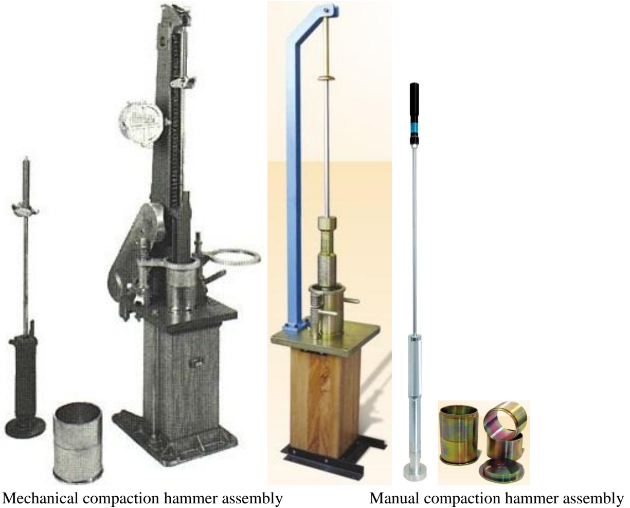
Figure 17.3 Pedestal, hammer and mold used in preparing Marshall test specimens
