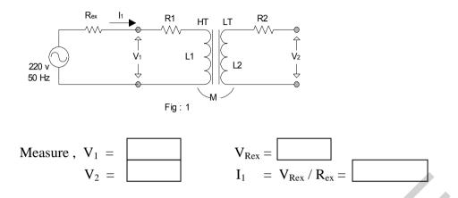
NB: Make sure that you connect the HT side to the supply and measure  $V_2$  across the end terminals of secondary side.
