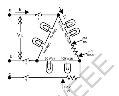
Observe the wave shapes of  $I_L$  and  $I_p$ . Take measurement of their phase difference: Which wave is lagging ?
