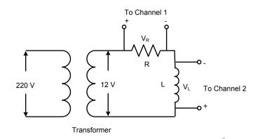
Figure 3: Experimental setup for R-L circuit
