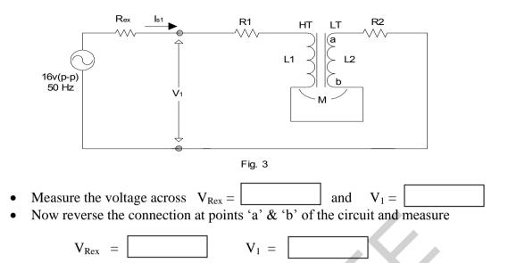
From these two readings determine which connection is for aiding and which one is for opposing flux. Mark the terminals of the transformer with appropriate dot notations.
