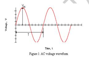
Here, Time period = T, Frequency  $f = \frac{1}{T}$  $v(t) = V_m \sin(2\pi f \cdot t)$ ,  $V_m$  or  $V_p$  = peak value =  $\frac{V_{p-p}}{2}$
