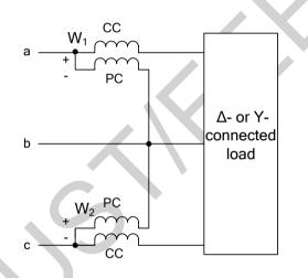
Figure: Two-wattmeter method for  $\Delta$ - or Y-connected load.
