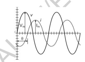
Figure 2: Phase difference between a voltage and a current waveform.
