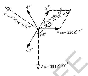
Figure: Line and phase voltages for a-b-c sequence.
