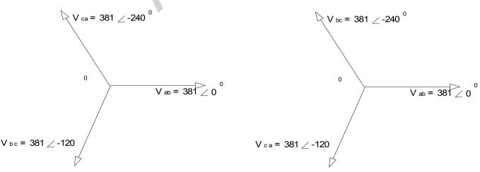
Fig: 4 Line to Line voltages for 'ab-bc-ca' sequence
