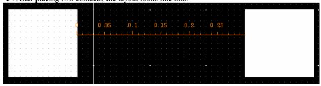
8. Now, contact to oxide spacing is minimum 0.06  $\mu$ m. So, draw a rectangle of 'Oxide (drw)' layer so that it covers both the contacts and extends from each side by 0.06  $\mu$ m. While drawing this, you will see Design rule violations when they are committed.
