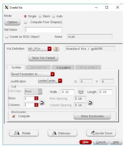
**19.** Also draw a 'Metal1 (drw)' rectangle on the via, because the default Metal1 rectangle area is less than the required minimum.
