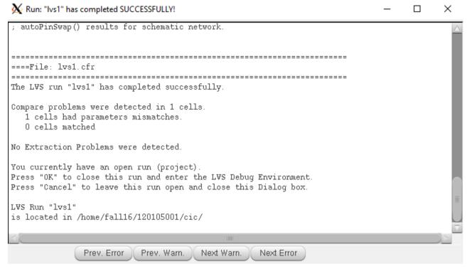
Note that, LVS report says that 1 cell had parameter mismatch. That means one cell had two different dimensions in schematic and layout. Click **OK**. 'LVS **Debug**' window will appear:
