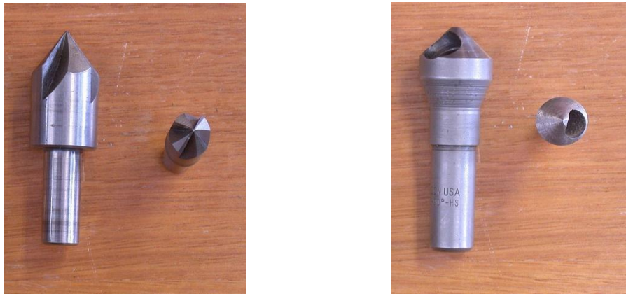
Figure 3.11: Countersinking cutters (4-fluted and non-fluted)
