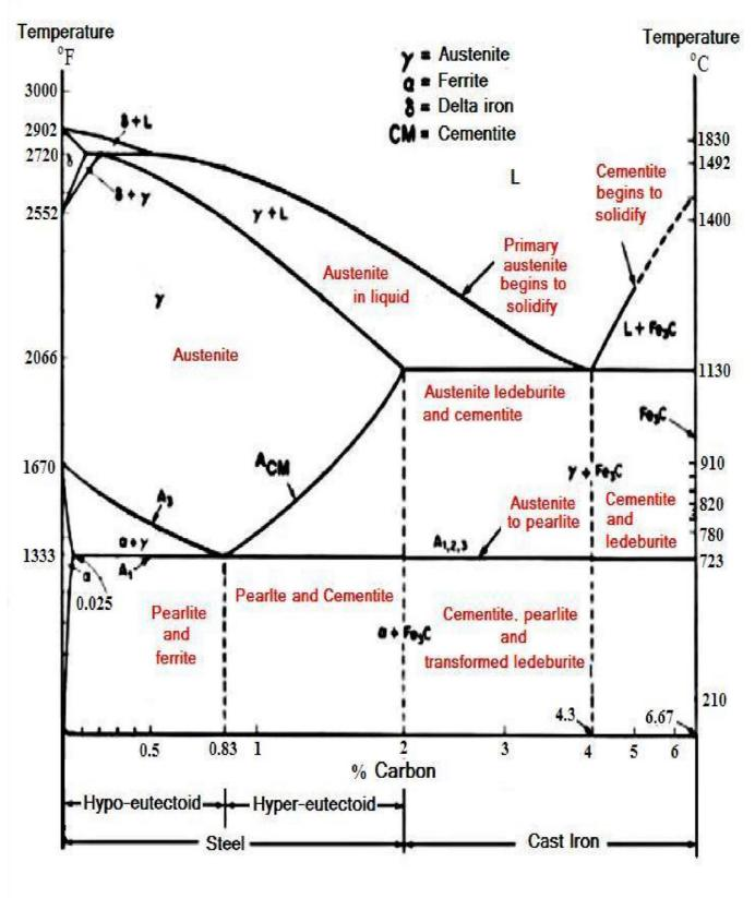
The Iron\_Iron Carbide (Fe\_Fe3C) Phase Diagram
