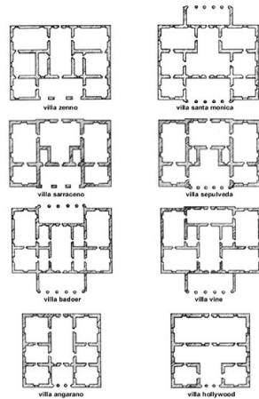
Figure 5- Possible Palladian villa plans after the Palladian villas grammar. (Stiny and Mitchell, 1978)
